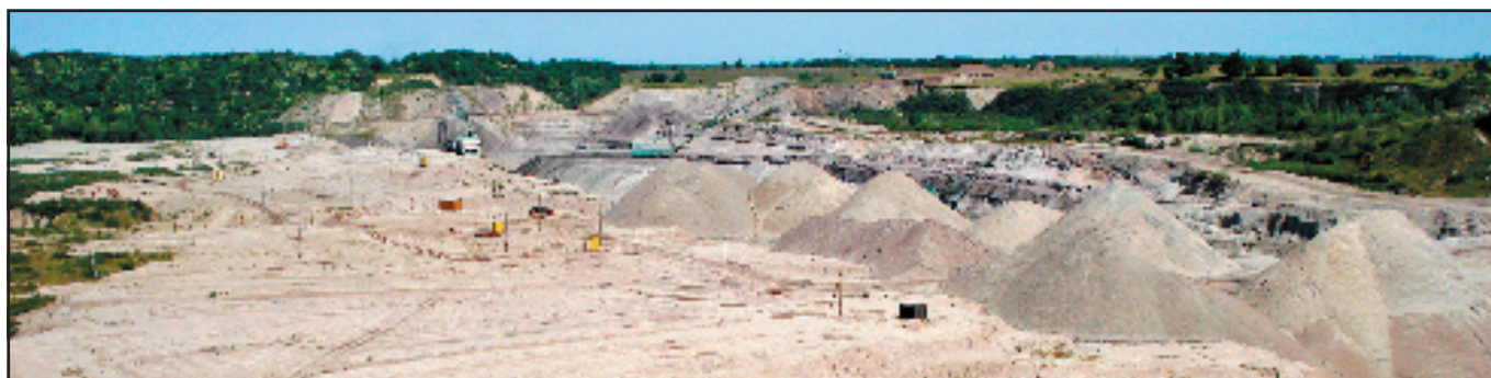
Current working in the Plazhovaya amber quarry at Yantarny, with three draglines along the main face that is partly hidden by the spoil heaps of overburden.
